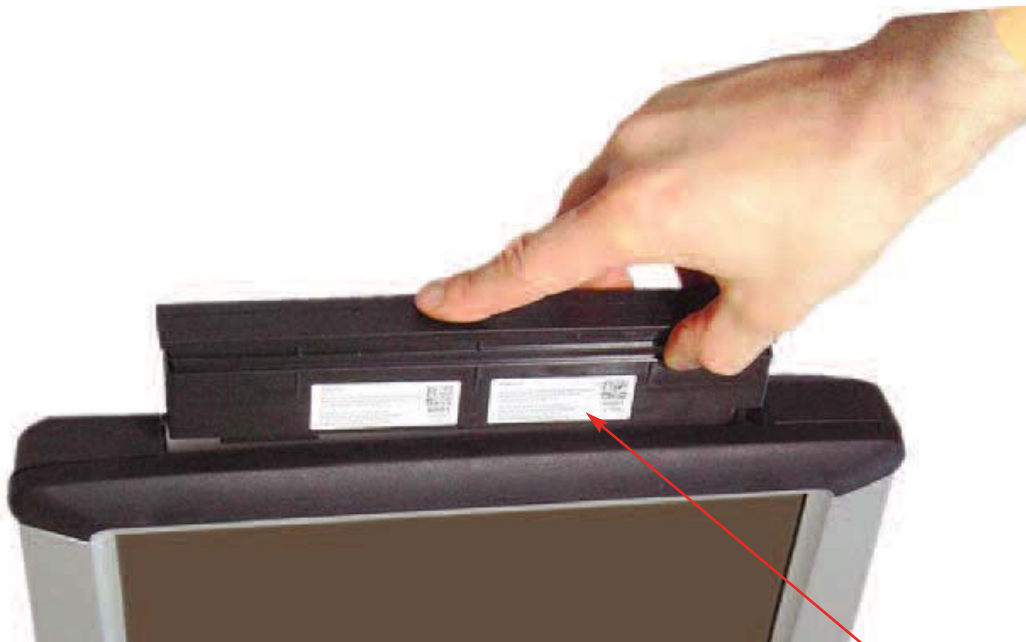
Inserting the rechargeable battery pack
